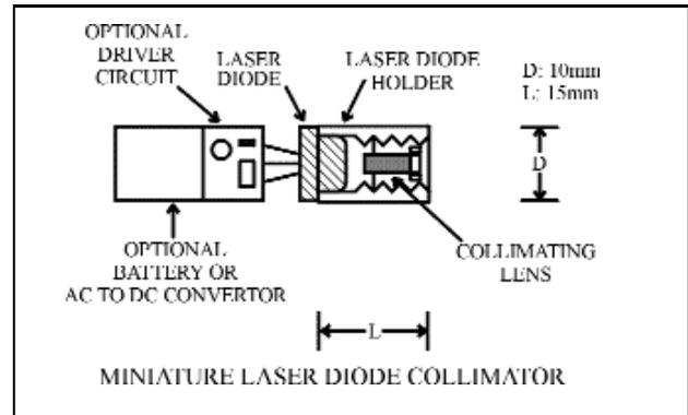
Laser diode collimators are used to collimate the highly divergent beam that is emitted by a laser diode. It consists of a laser diode holder, a collimating lens holder, and a high numerical aperture (NA) collimating lens, with a focal length  $f$ . The lens is housed in a threaded receptacle that is screwed into the collimating lens holder. By adjusting the distance between the laser diode and the collimating lens, one can collimate the laser diode output.
