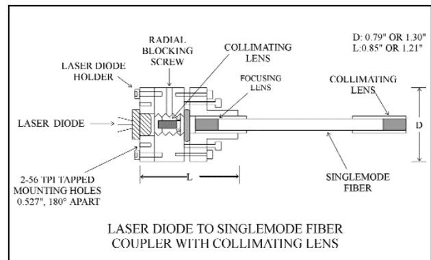
OZ Optics also offers special compact laser diode to fiber couplers for OEM applications. These packages have the diode and collimating lens permanently glued into the same housing. This package features a compact, rugged housing, at a significant reduction in cost.
